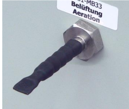
Fig. 6: Hose nozzle of the aeration valve with heat shrink tube (example illustration)
