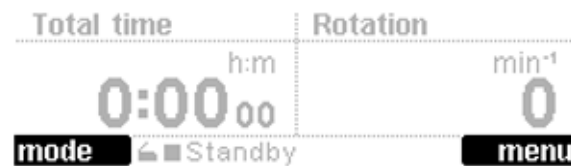
Fig. 22: Display of the assignment of the function keys; here: left key "mode", right key "menu"
