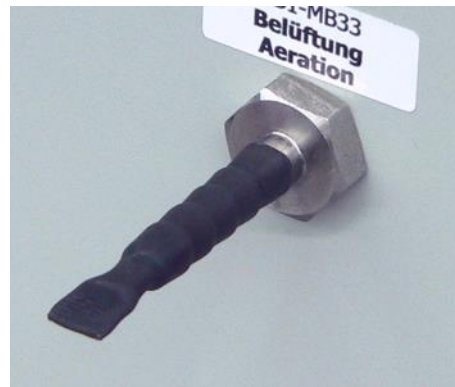
Fig. 7: Hose nozzle of the aeration valve with heat shrink tube (example illustration)
