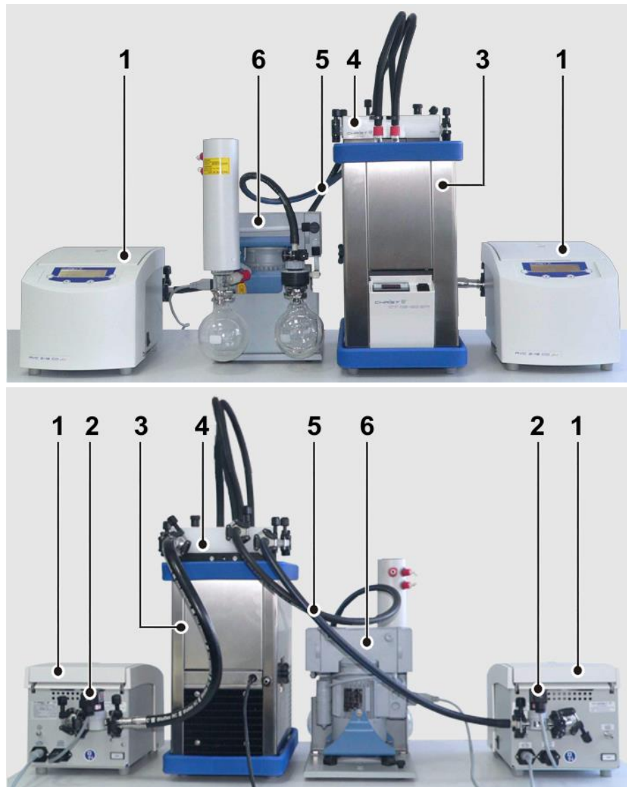
Fig. 14: Combination of two RVCs with a vacuum pump and cooling trap with a distributor block, front and rear view
