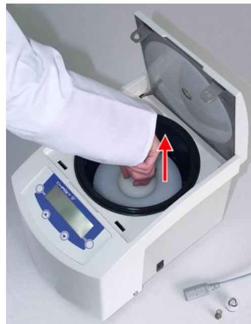
Fig. 47: Removing the rotor shaft
